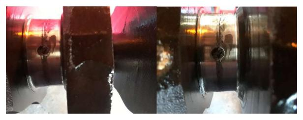
Grime all over bushings and the scoring it caused on the rod ends from lack of oil.
