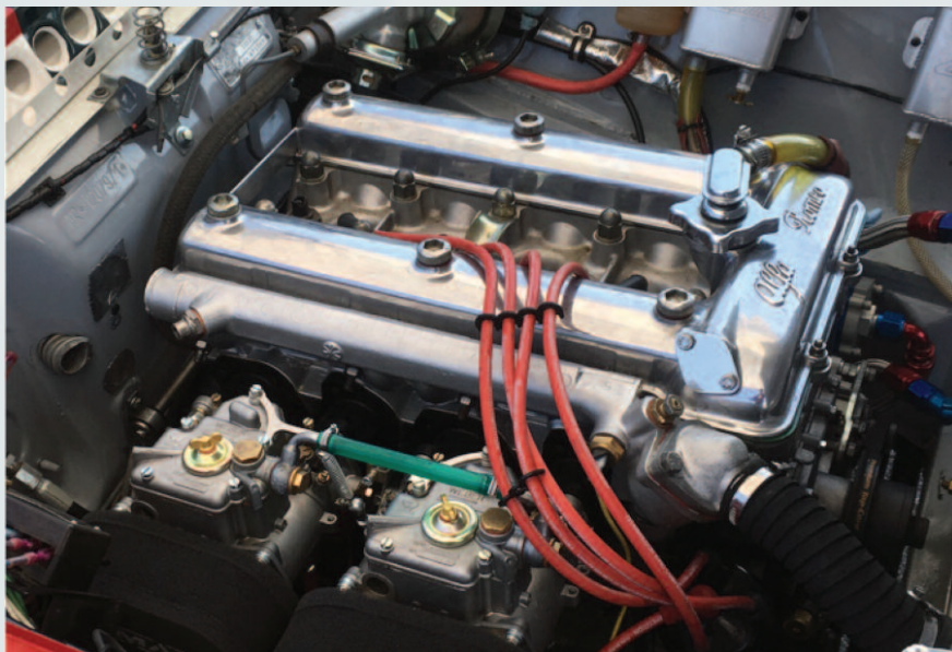
Figure 2. Weber carburetors in a well-prepared Alfa race car.
