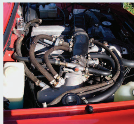
Figure 4. Series 3 Spider Jetronic fuel injection system.
