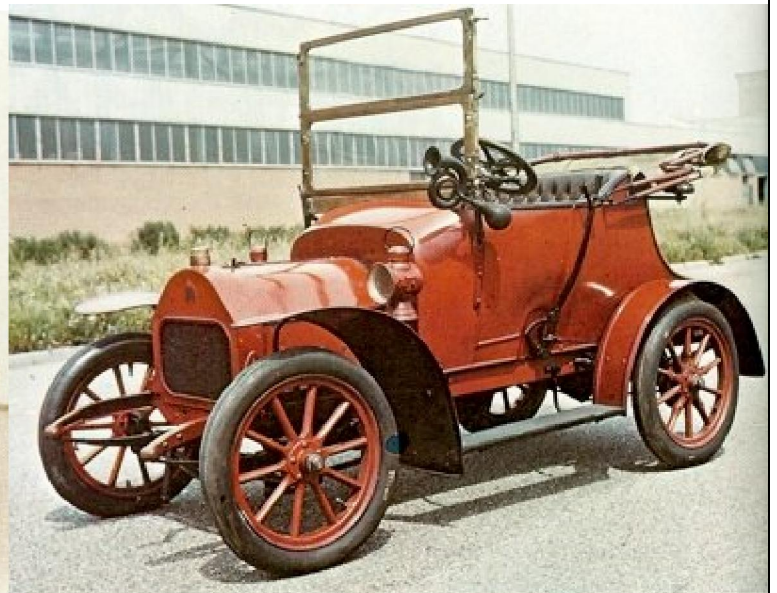
1908 8/10hp Darracq, which was fitted with an 1100cc single engine.
