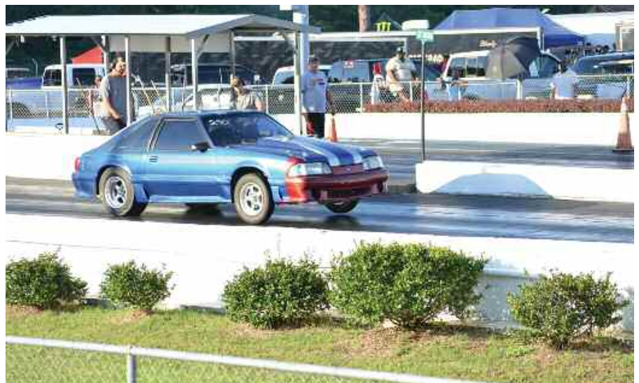
Figure 3: A modern drag racer displaying the lifted front end and twisted chassis that results in left front wheel lifting off of the racing surface.
